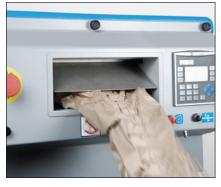
The PadPak® LC is the fastest paper cushining solution on the market. The high output allows a maximum box throughput. The converter forms single layer paper into pads which can be used to protect products during shipment. The individual fanfolded
