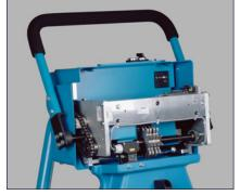
The mobile PadPak® JR converts two layer paper into exceptional cushioning pads which can be used to protect products of all shapes and sizes during shipment. The paper pad has an incredible shock absorbing capacity. By using this
